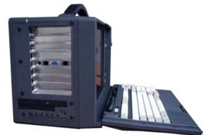
6 PCI slots enable complex applications
