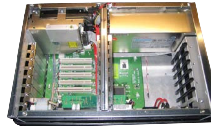
6 PCI slots enable complex applications
